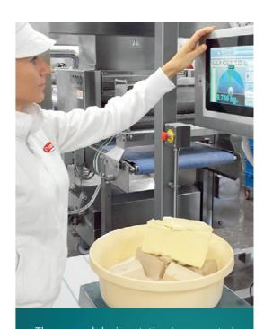
The manual dosing station is connected to the automation system. Dosing report is saved to database for quality control.
