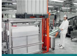
The dosing of fluids like syrup and malt extract can be automated with the Fluidmatic™ dosing unit. This compact solution is reliable and space-saving.
