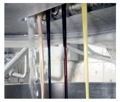
A typical raw ingredient system for a medium sized commercial bakery consists of, for example, 2 silos (rye and wheat flour), 6-8 Big Bags, 10 small ingredients, 2 sourdough starters and a few fluids. Depending on the system dimensions, the system will automatically and with a high degree of precision dose 10-15 medium-sized (300 l) dough batches an hour. A single person can easily manage the entire dough production process.
