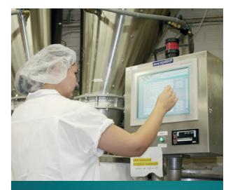
Automatic recipe dosing is started by selecting the right recipe from the menu and then pressing the Start button. A single person can easily manage the entire dough production process.
