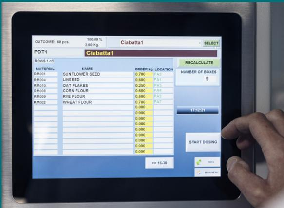
▲ RECIPE-CONTROLLED DOSING WITH A USER-FRIENDLY OPERATING INTERFACE. EQUIPPED WITH A DATABASE AND A PC LINK FOR QUALITY CONTROL.
